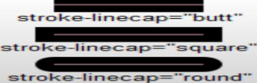
The diagram shows three horizontal bars. The top bar is a simple rectangle labeled `stroke-linecap="butt"`. The middle bar is a rectangle with a small vertical extension at its right end labeled `stroke-linecap="square"`. The bottom bar is a rounded rectangle labeled `stroke-linecap="round"`.
